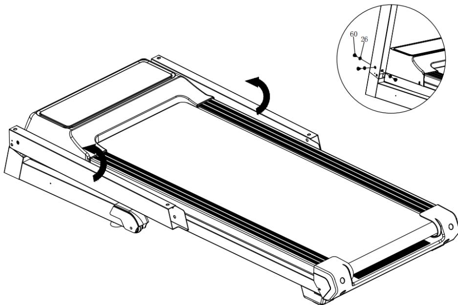
**STEP 3:** Connect the cables between the console and the right front support (16R) and fasten the console to the front supports with M8\*16 screws (60) and washers (26) (tighten all screws firmly).
