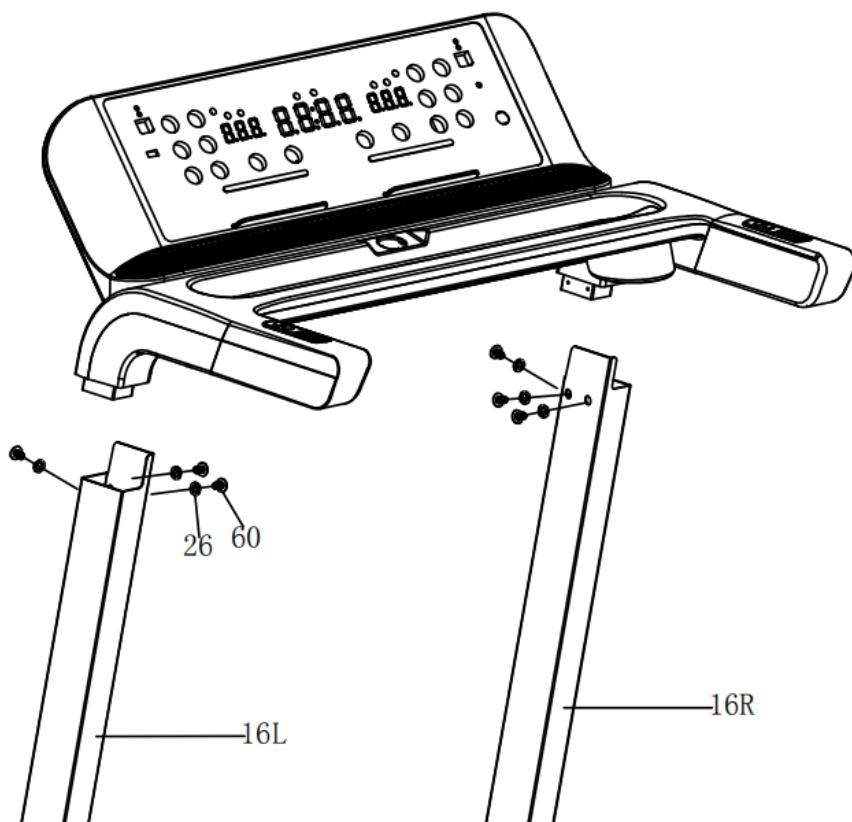
**Step 4:** Use the supplied M4.2\*16 screws (3) to secure the cover firmly to the front supports (16L/R).
