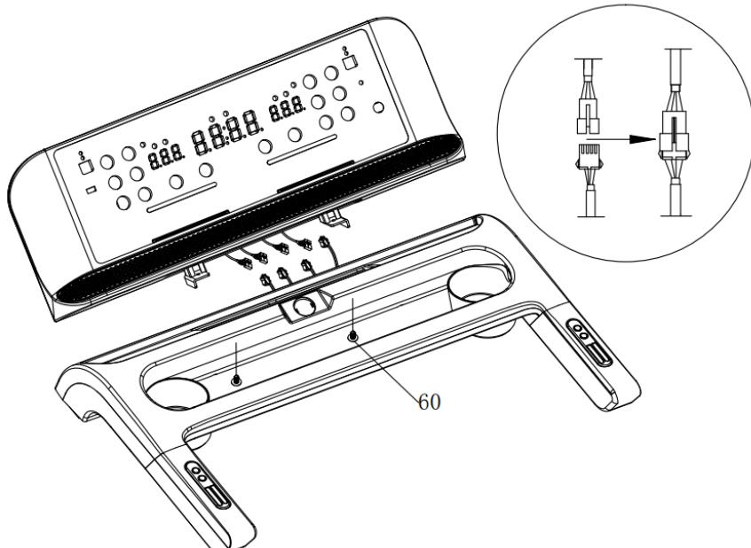
**STEP 2:** Place the main frame on the floor. Lift the front supports and use the supplied M8\*16 bolts (60) and washers (26) to secure them to the main frame (do not tighten the bolts).
