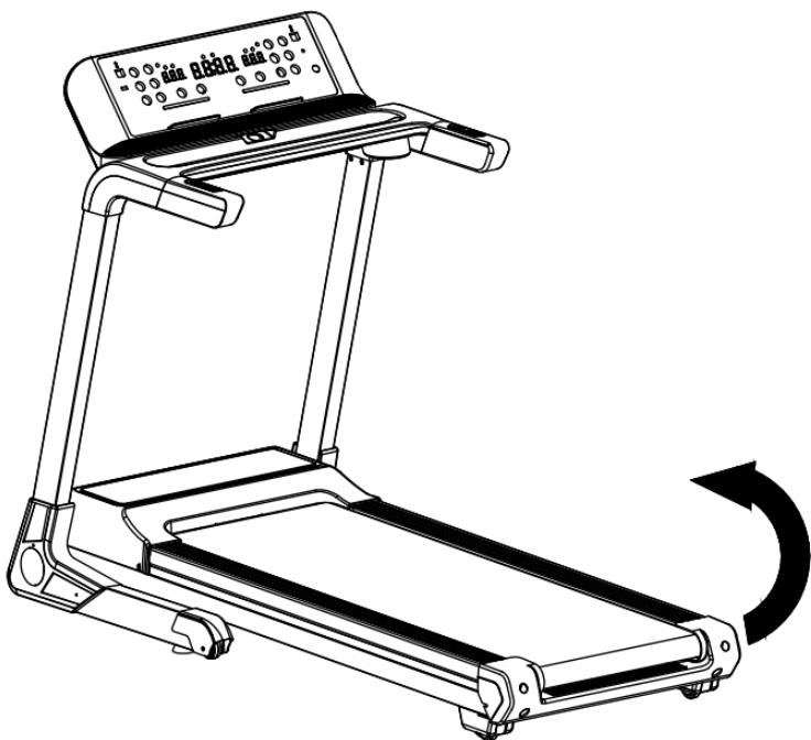
Lift the tread and pull it up with force until you hear a "click" and feel that the safety mechanism is engaged.
